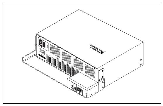
Figure 10. Rear Guard Installed on the MID-7654/7652
